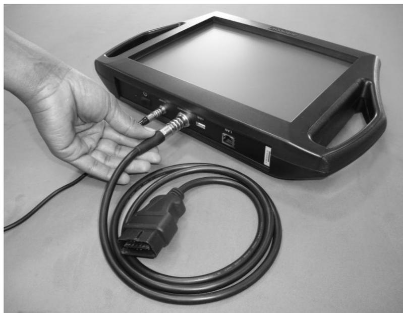
4. Connect the other end of the diagnostic cable to the vehicle's diagnostic socket.
