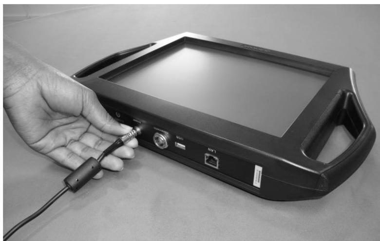
2. Select the correct diagnostic cable for the vehicle you are working on.
